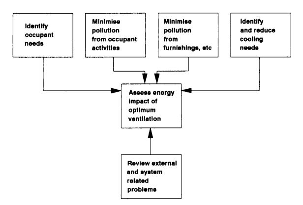
Figure 5: Optimum ventilation needs
