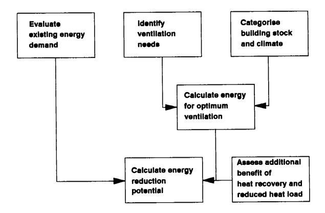
Figure 6: Achieve energy and cost effective ventilation - system design needs
